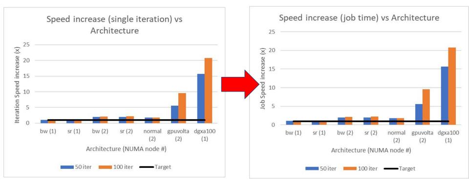
\*Normalised against 1 NUMA node normalsr calculation sr = Sapphire Rapid, bw = Broadwell, gpuvolta = V100, dgxa100 = A100
